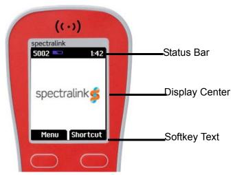
The display is divided in three parts: **Status Bar**, **Display Center** and **Softkey Text** (see figure above).
