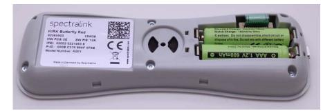
1 Press the back cover in locked position (when you hear a click, the back cover is in position). Use only Ni-MH rechargeable batteries.
